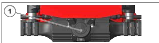
Illustration 121: Kontrollér forakslens differentiale for lækager
